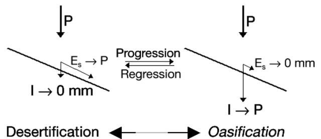
**Figure 1.** *Oasification* against desertification. P: precipitation.  $E_s$ : surface runoff. I: infiltration.
