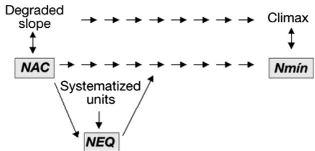
**Figure 4.** Progressive series of the curve number (Martínez de Azagra, 1996).  $NAC$ : curve number on the actual slope.  $N_{min}$ : end curve number on the restored slope.  $NEQ$ : equivalent curve number on the systematized unit.
