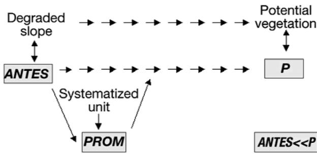
**Figure 5.** Progressive succession of infiltration and available water on a degraded slope (Martínez de Azagra, 1996). ANTES: available water for the slope without primary systematization. PROM: average available water for the systematized units. P: quantity of rainfall.
